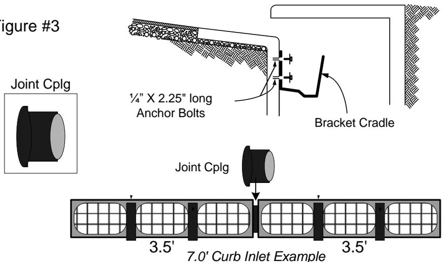
**Note:** To secure Curb Inlet Filter in place, fasten zip ties to Cradle Bracket and Curb Inlet Filter as shown.
