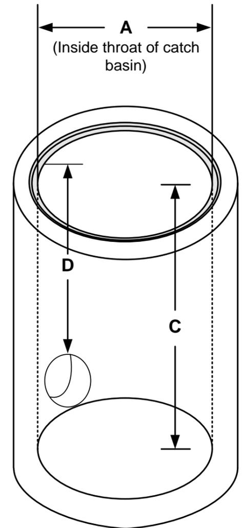
**Sizing Guide for Square Drop Inlet Catch Basins
