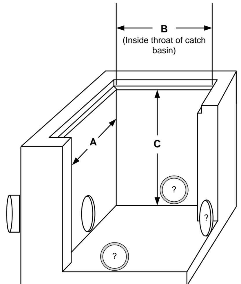
**Sizing Guide for Round Drop Inlet Catch Basins**
