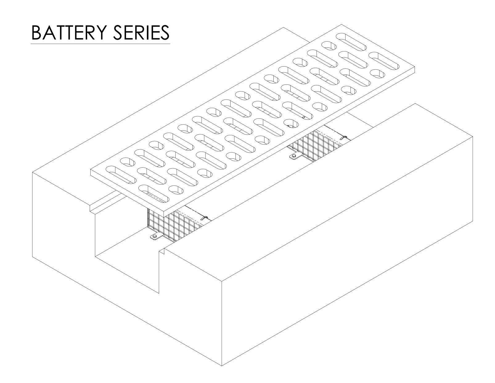
T-DAM SHOWN IN BATTERY SERIES, WITH TWO UNITS WORKING IN UNISON TO OPTIMIZE FILTRATION.
